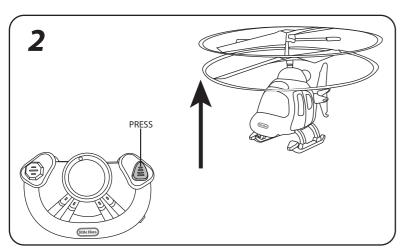
Press the TAKE OFF button to make the helicopter fly upward to height level 1. Press the button again to elevate the helicopter to height level 2, and then it will go back to height level 1 after five (5) seconds.
