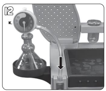
Fit the long end of the gauge tubing (K) into the air pump. Place the short end of gauge tubing into the flask and set the flask on the flask holder.
