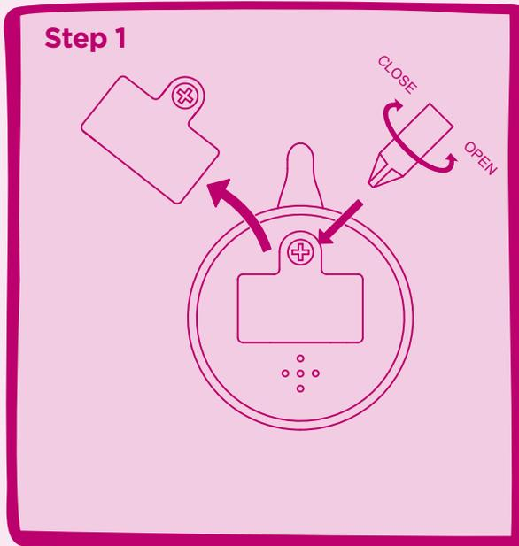
Open and close the battery cover with a screwdriver. (Philips screwdriver not included)
