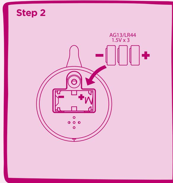
Install 3 x AG13 (LR44) 1.5V batteries and follow the polarity as shown.
