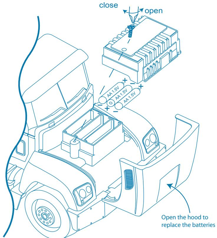
Open the hood to replace the batteries
