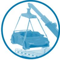
TOWING HARNESS CONNECTS TO CAR AND CRANE HOOK
