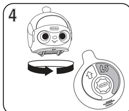
Press the right arrow to turn the RC car in place.
