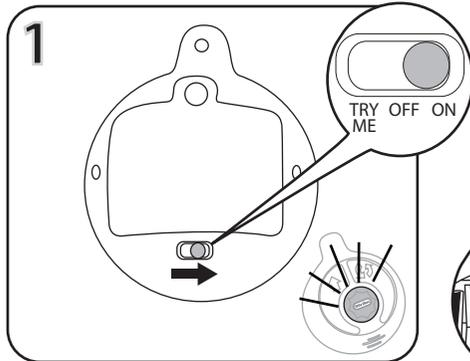
Move the switch on the back of the controller to the ON position. The light on the center button of the remote will flash.
