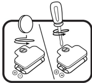
4. Install 2 new AA (AM-3/LR6) and 3 new AAA (LR03/AM-4) batteries following the diagrams inside each battery box. (For best performance, alkaline batteries or fully charged Ni-MH rechargeable batteries are recommended).
