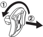
① Rotate the 3 packing locks counterclockwise 90 degrees.
